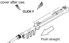
Be careful not to slant SC connector while inserting into the Guide cap.
