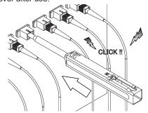
Be careful not to slant the Cleaner SC while inserting into the adapter.
